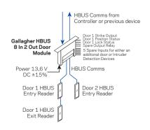
HBUS entry and exit readers connected to the Gallagher HBUS 8 In 2 Out Door Module for the access control of one door.
